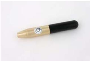
**Mini pig transmitter „A“**, water-proof (16 bar) pig transmitter for the exact determination of the end-point of the glass-fibre rod, detectable up to approx. 5 m depth. Frequency „A“ resp. 42 kHz, approx. 10 h operating time.
