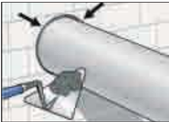
1 - Seal the fissures around the pipe with mortar.
