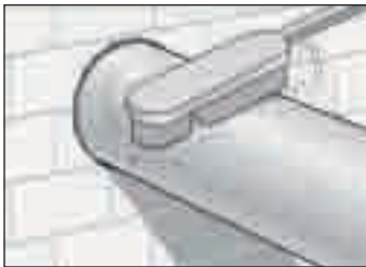
2 - Clean the pipe before applying the fire resistant sleeve.
